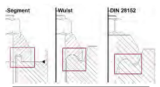
The different between the segment screw clamp and the Wulst/DIN 28152 screw clamp is the contact surface and its geometry.
